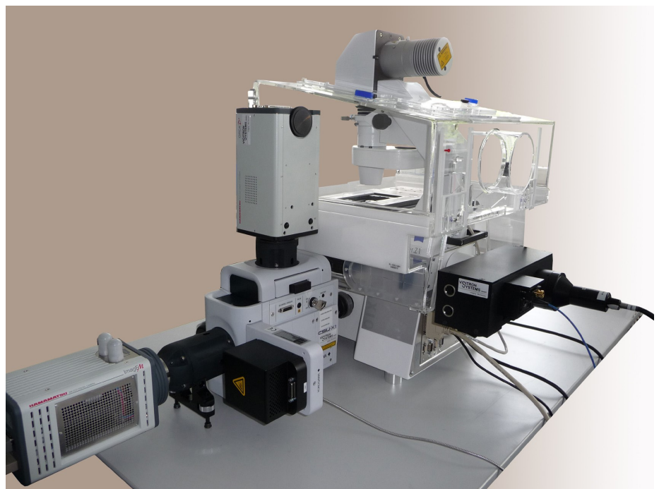
Zeiss Axio-Observer with 2D FRAP, CSU-X1 with dualcam.
